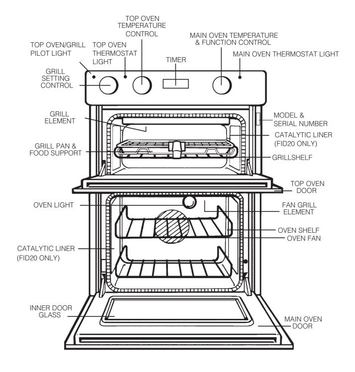
NEVER line the shelves, floor or sides of the oven or grill with aluminium foil as overheating and damage may result.
